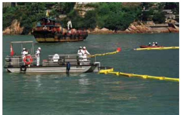
▲ Deploying oil containment booms to surround the polluted area 放置圍油欄圍繞受油污污染海面
