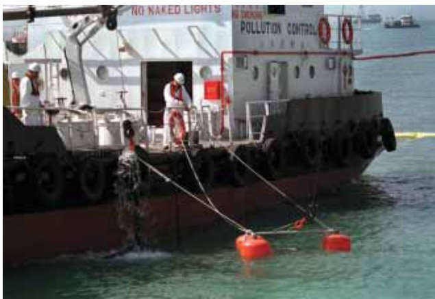
▲ Demonstration of oil recovery by skimmers 以撇油器將海面油污收回示範
