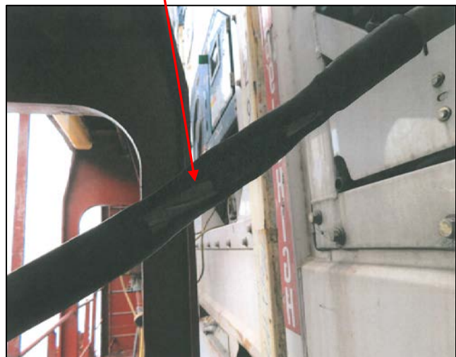
Torn reefer cable sleeve 冷凍貨櫃電纜套筒損毀
