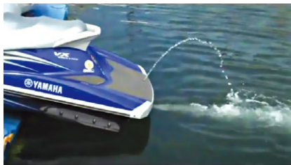
Cooling water tell tale 正常運水指示
