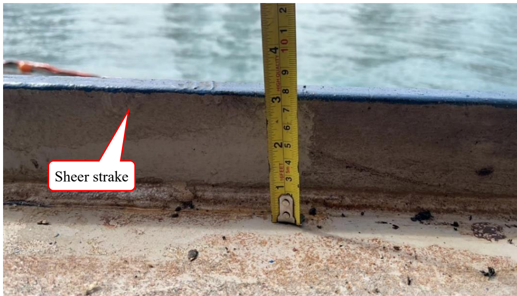
Figure 6: height of sheer strake
