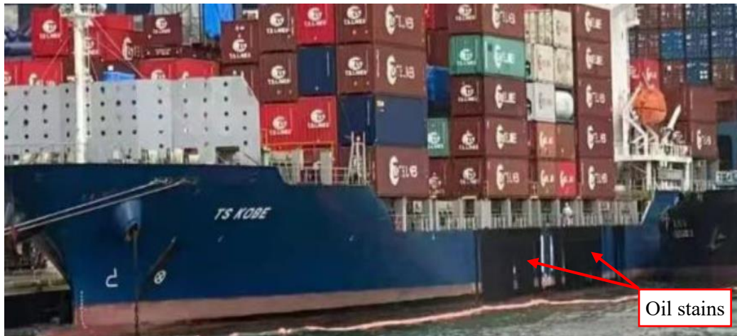
Figure 3: hull stained by the overflowed oil
