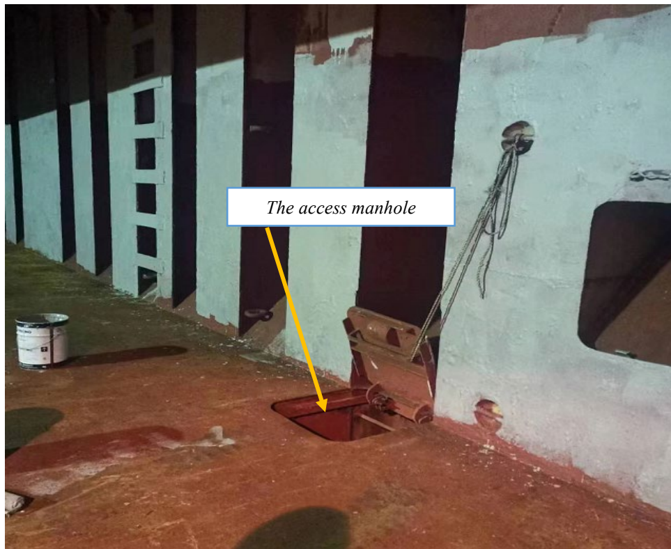
Figure 3: The access manhole located at the tween deck of the hold for access to/ from the lower cargo hold
