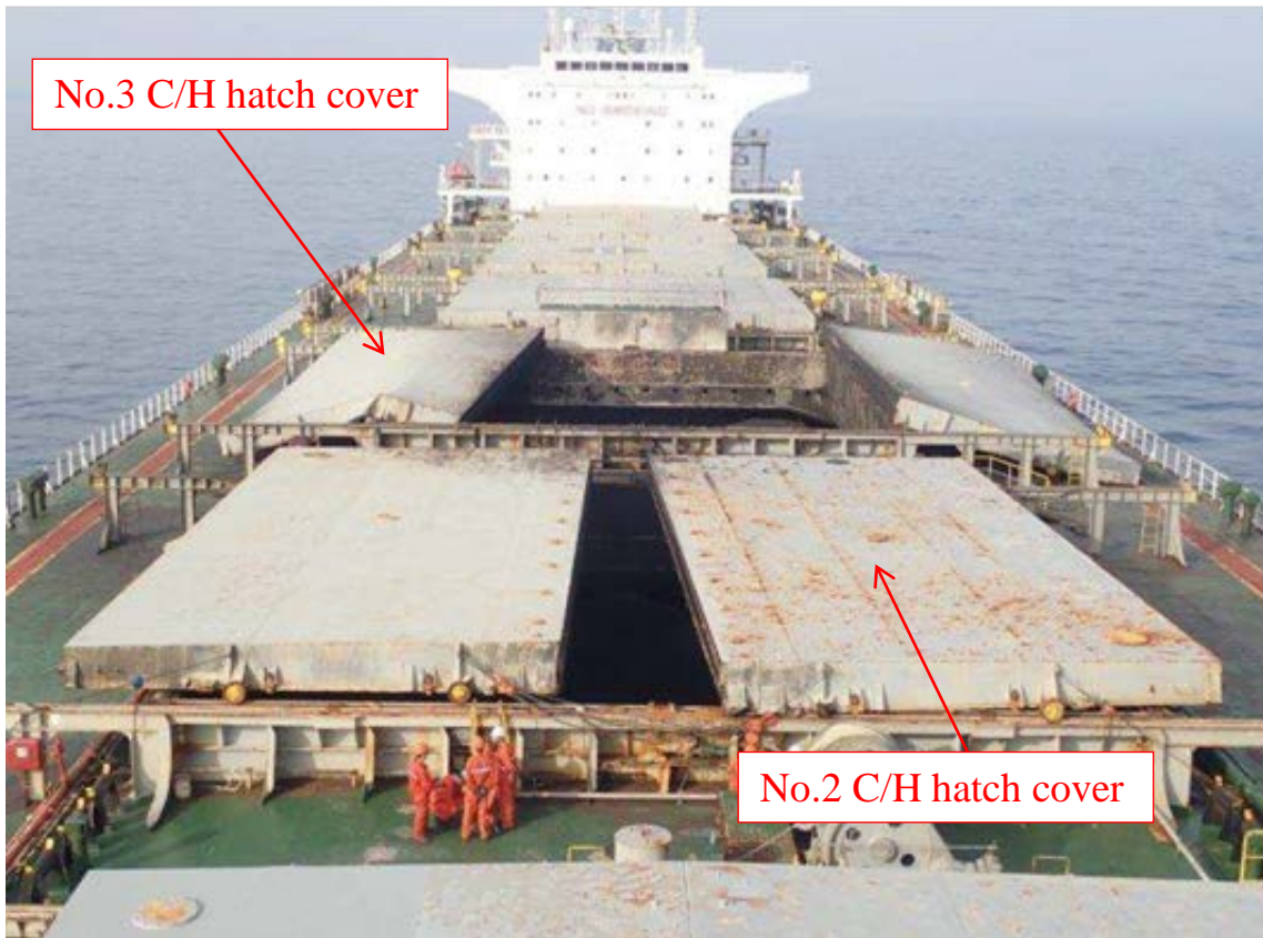
Figure 3 The dislocated No.2 and No.3 C/Hs hatch cover panels (looking aft)
