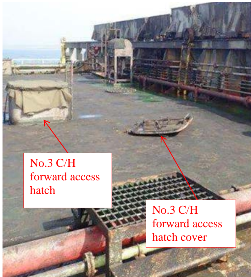
Figure 9 No.3 C/H forward access hatch and the dislodged cover
