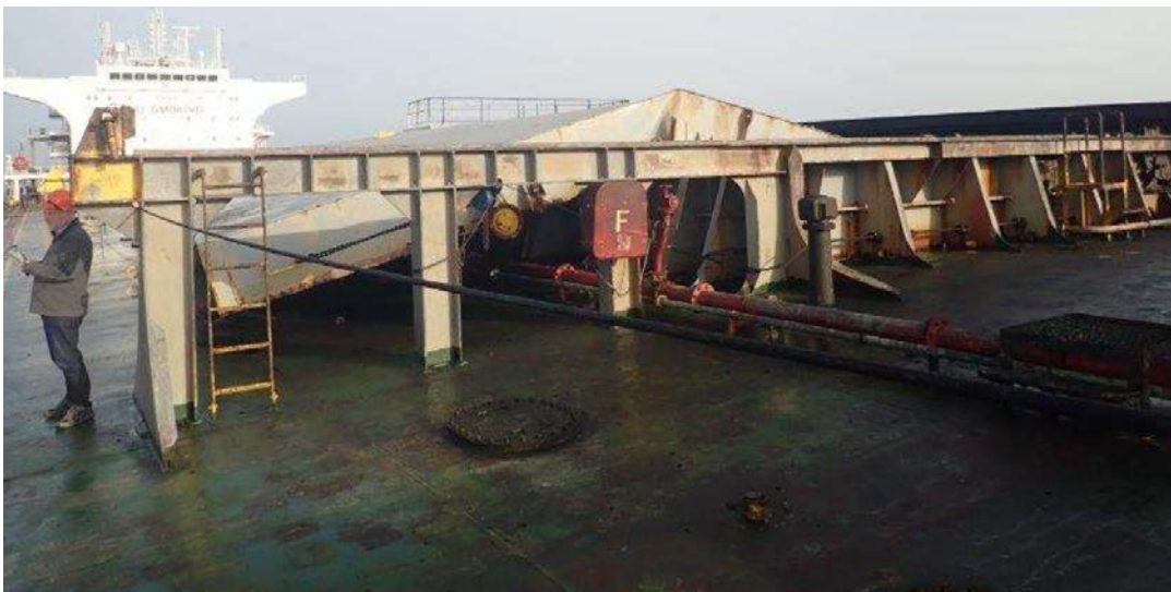
Figure 7 Forward end of No.3 C/H hatch cover starboard panel
