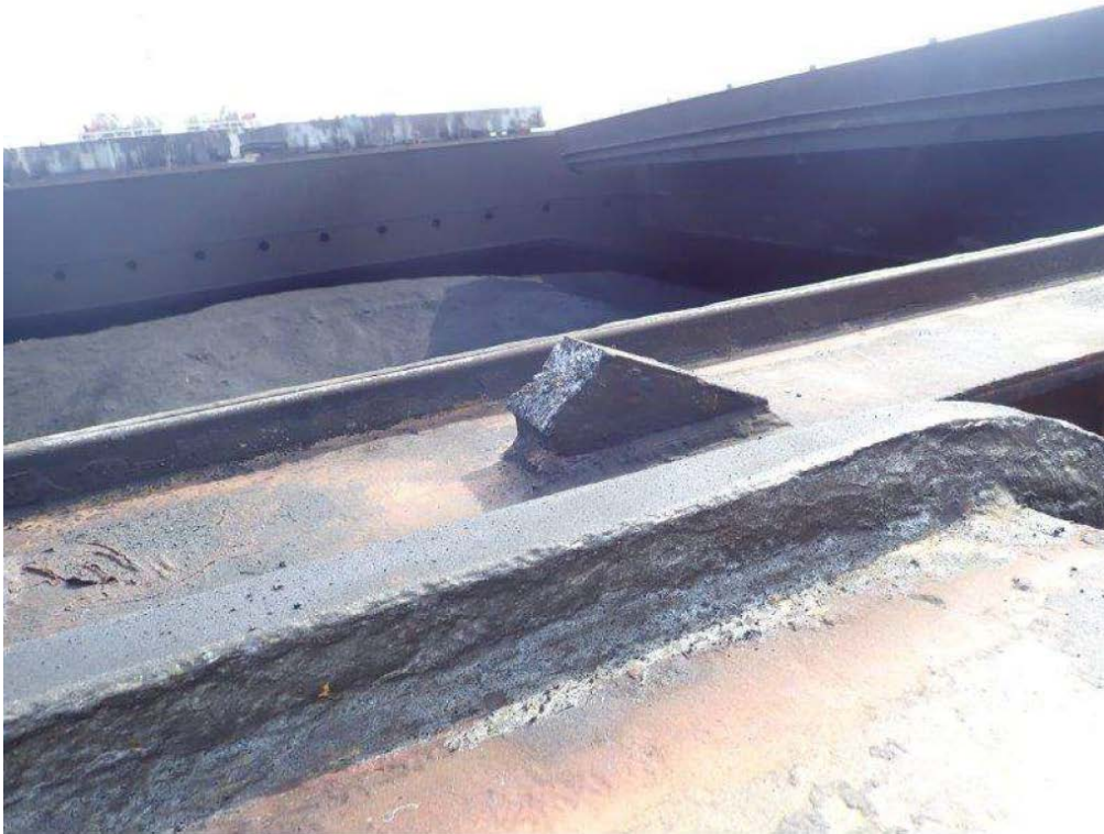
Figure 8 Broken No.3 C/H hatch cover securing cleat
