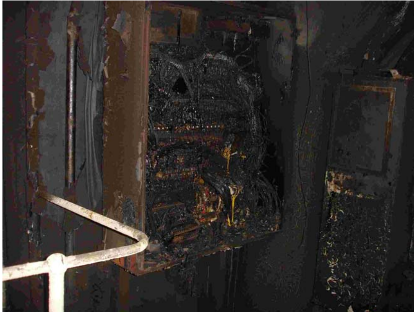
Fig. 15: Damaged Electric Distribution Panel in Engine Room
