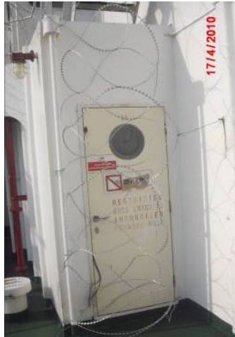
All accommodation entrances locked from inside and blocked from outside.
