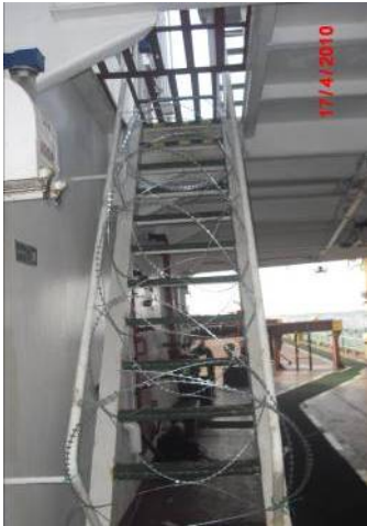
All accommodation entrances locked from inside and blocked from outside.
