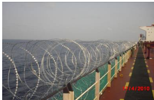
Barbed wire fencing completed all around vessel.
