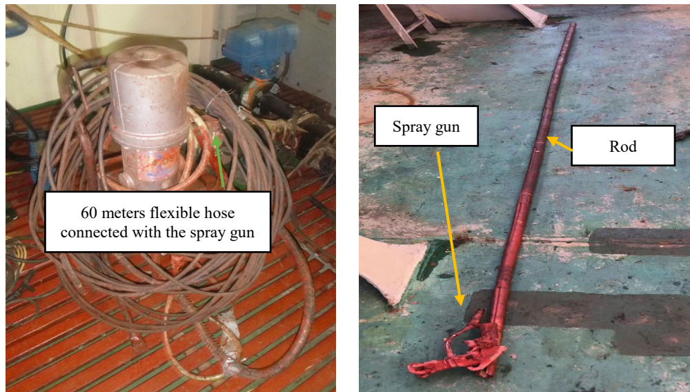
Figure 2: pneumatic sprayer machine and spray gun tied up with the rod
