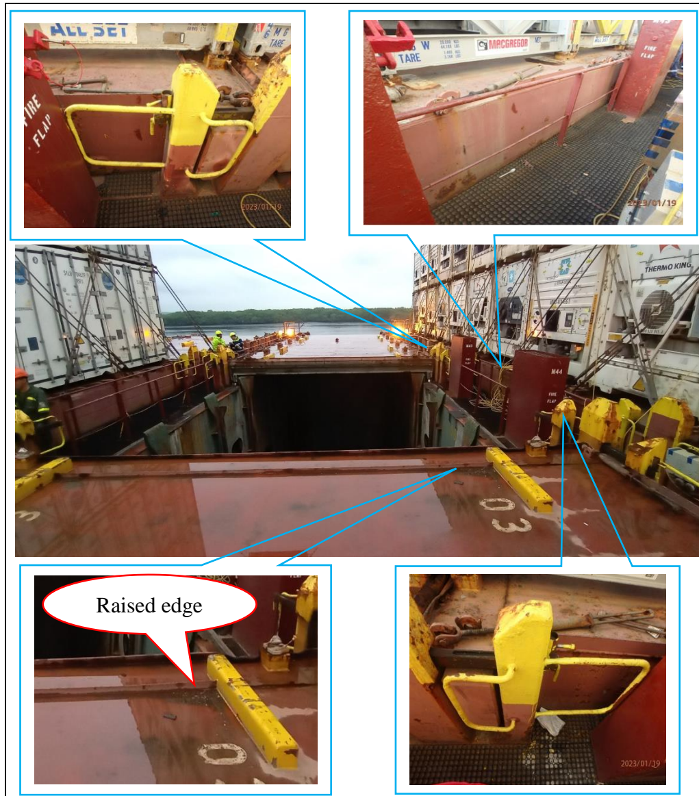
Figure 9: Conditions of catwalk, railings and hatch cover between bays 18 and 21
