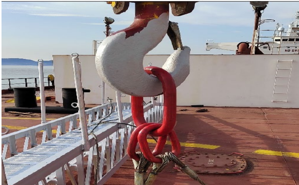
Figure 10: the manufacturer-qualified composite lifting unit of the portable gangway
