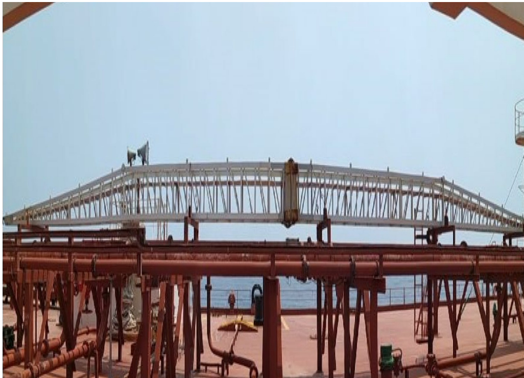
Figure 2: the portable gangway secured on the deck
