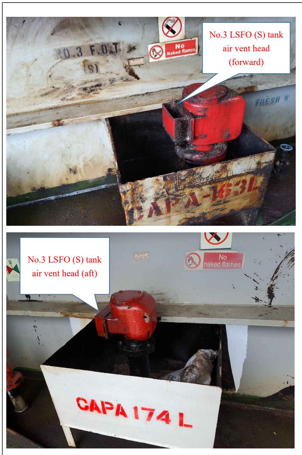
Figure 3 Oil spilled from the air vent heads of No.3 (S) LSFO tank
