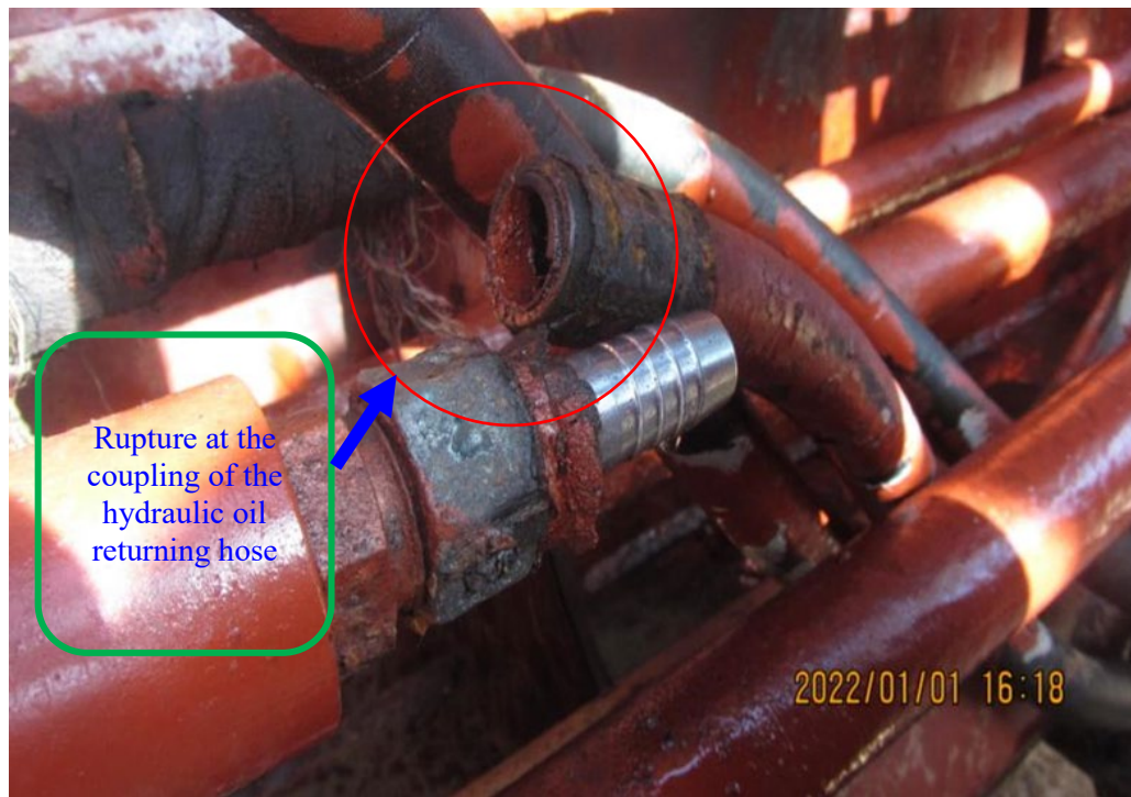
Figure 4: Rupture of the hydraulic oil returning hose
