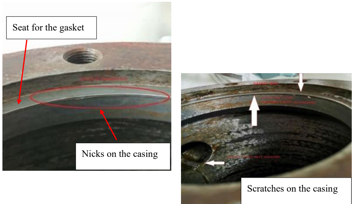
Figure 5 Minor damages on the casing of the filter .
