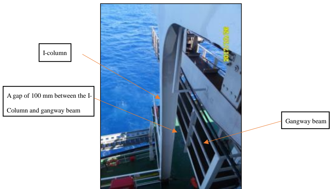
Figure 7 A gap of 100mm between the I-column and gangway beam
