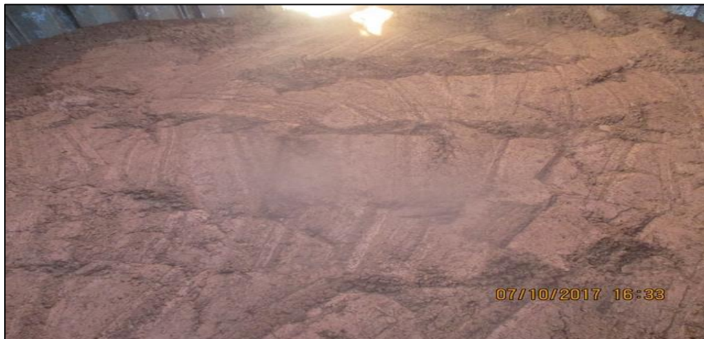
Figure 2 The cargo surface of one of the cargo holds after trimming
