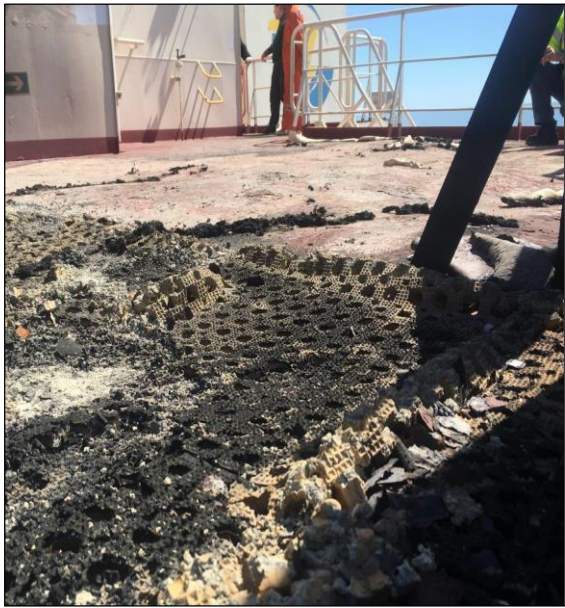
Figure 5 Burnt out of bridge wings
