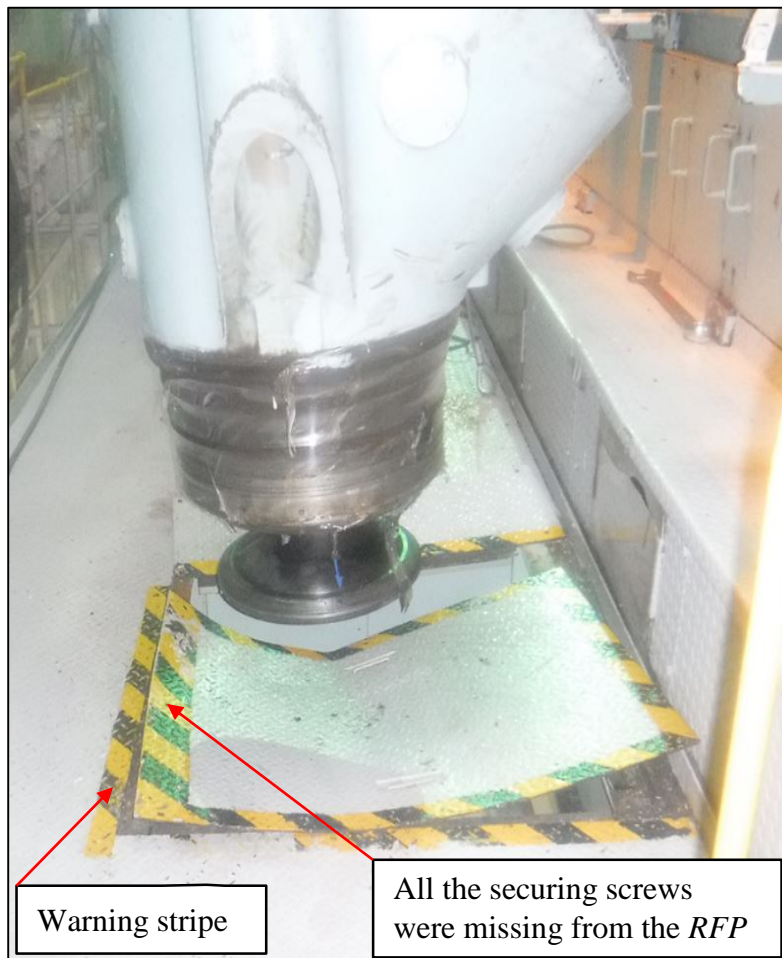
Figure 5: The deformed RFP with exhaust valve illustrated on it
