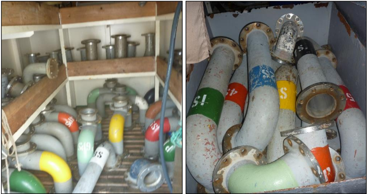
Fig. 15 - Elbow spool pieces for manifold connection.
