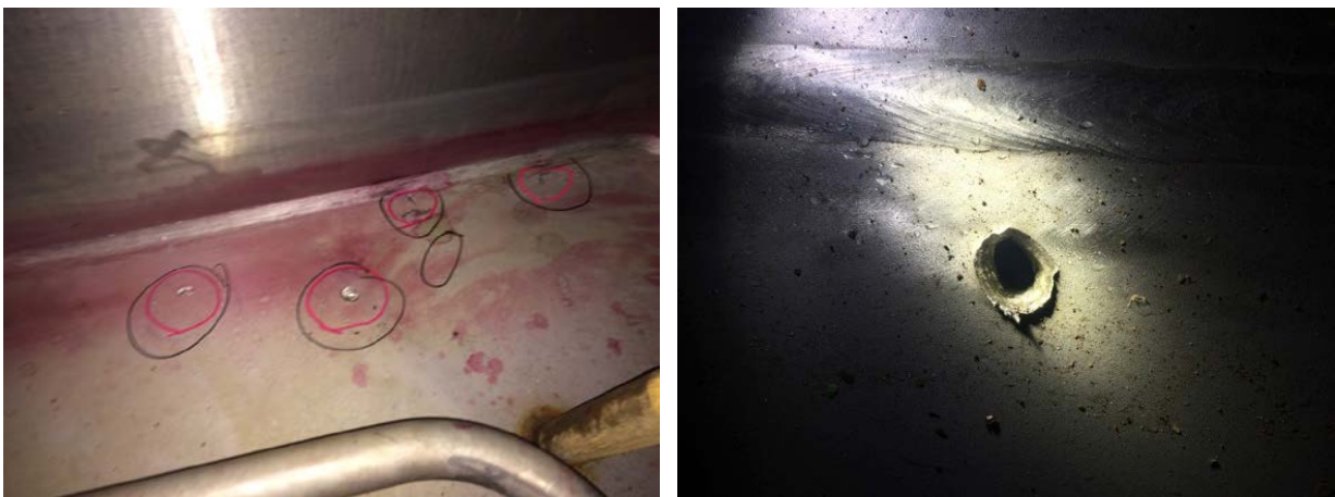
Fig. 9 – Pitting damage on bulkhead and bottom plate of COTs No.5 P&S
