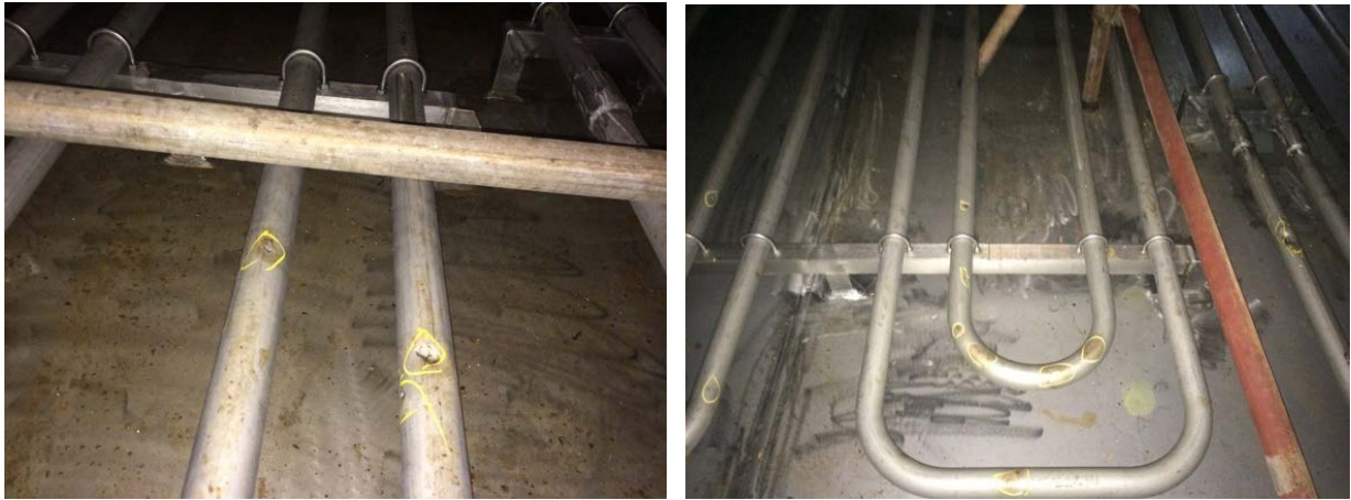
Fig. 8 – Damage on heating coils of COTs No.5 P&S
