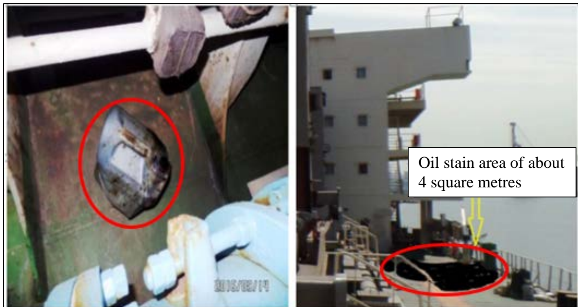
Figure 3 –the toppled fuel oil sampling bottle and the sketch map of the oil stain location on the main deck
