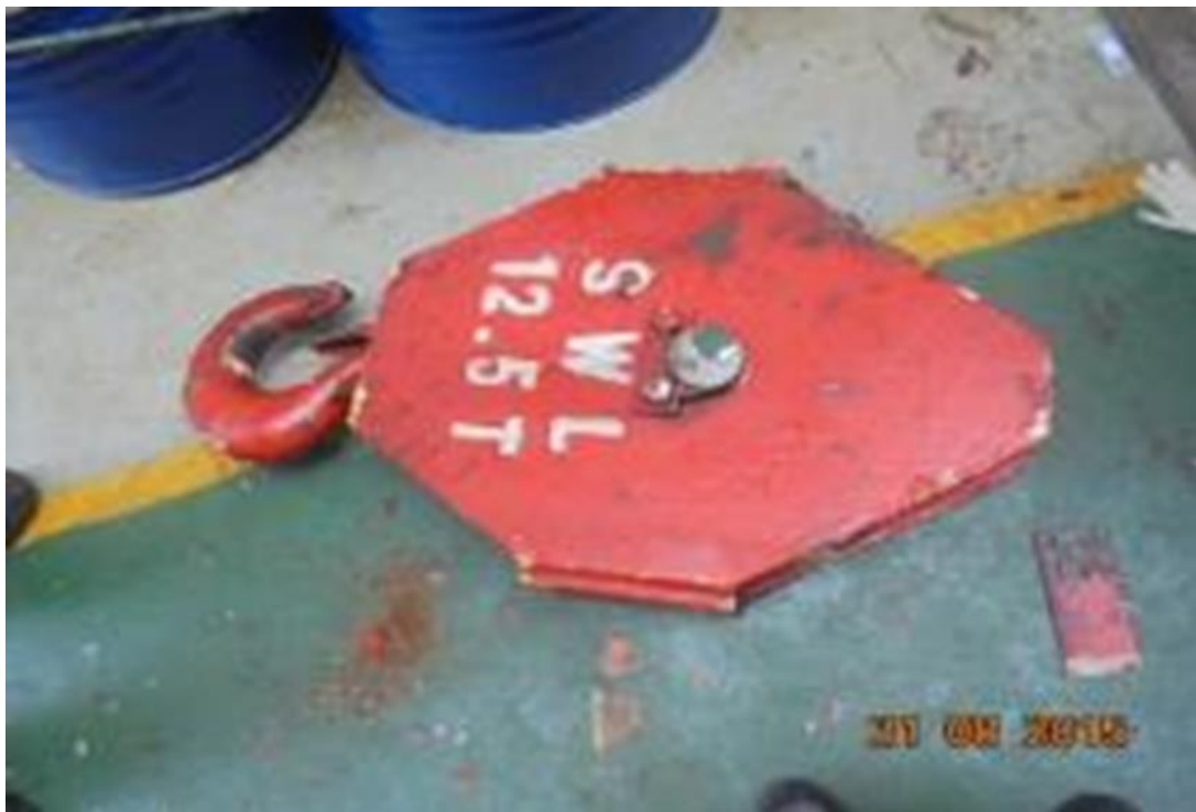
Fig.4- The hook block fell down on the deck
