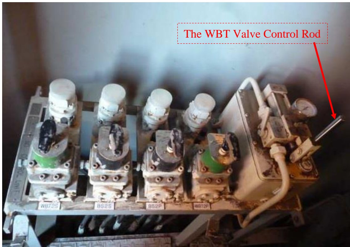
Fig.5- Beside the vertical ladder, the water ballast tank valve control block located on the bottom of the access trunk of the No.2 ship crane.
