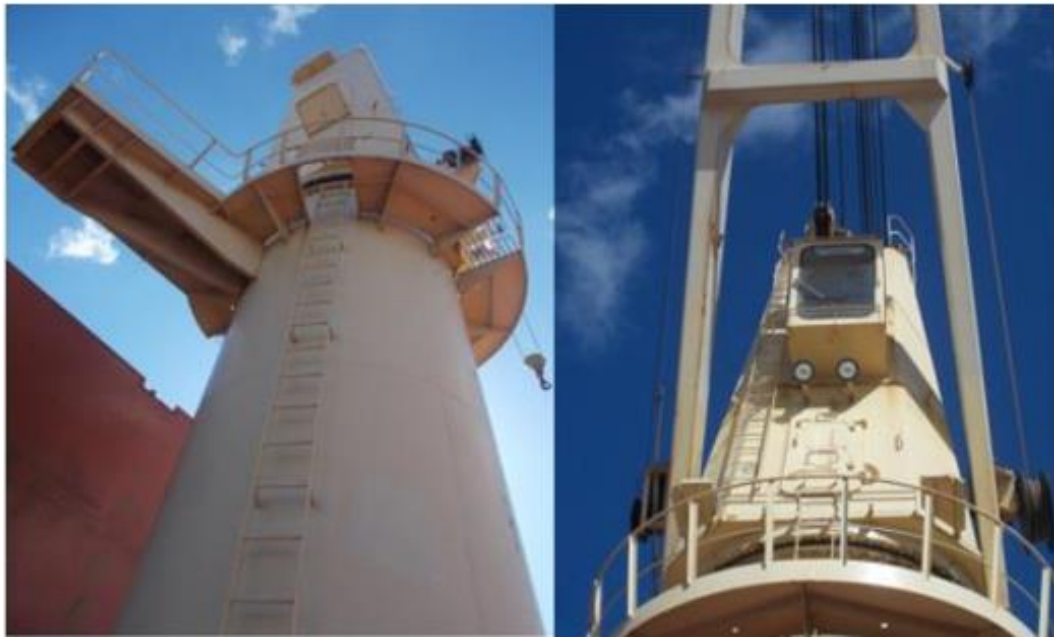
Fig.4- The vertical ladder outside and the driving cabin of the No.2 ship crane
