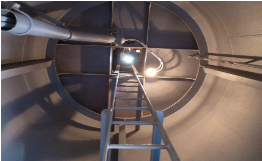
Fig.2 - The vertical ladder inside the trunk of No.2 ship crane
