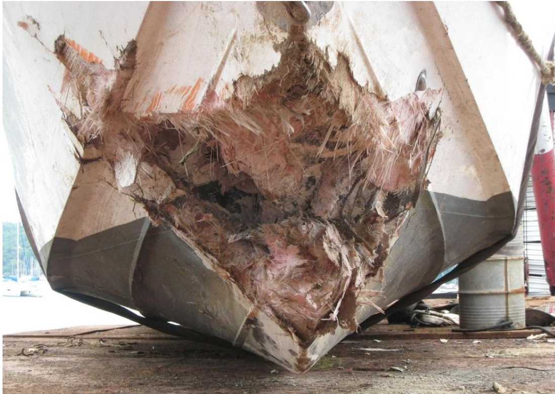
Fig. 4 - The damage of NAA-3797 at the bow
