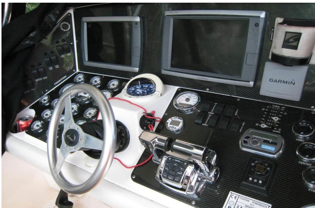
Fig. 6 – The safety lanyard and the toggle safety switch were intact after the accident
