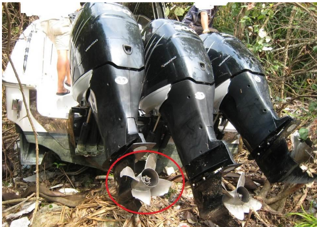
Fig. 5 – The propeller and skeg of the port outboard engine was damaged
