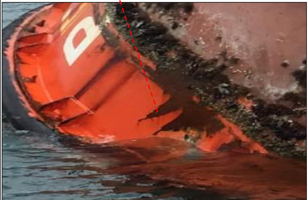
Fig. 12 – Fresh paint scratch and dent on the mooring buoy
