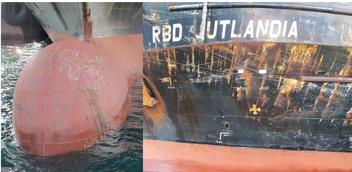
Fig.11 - Fresh scratches were found on the bulbous bow and port side hull of “RBD Jutlandia”
