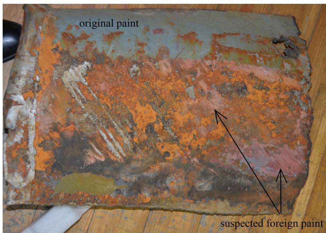
Figure 10 - Sample of steel plate cut from hole of the sunk Zhe Sheng Yu 05885
