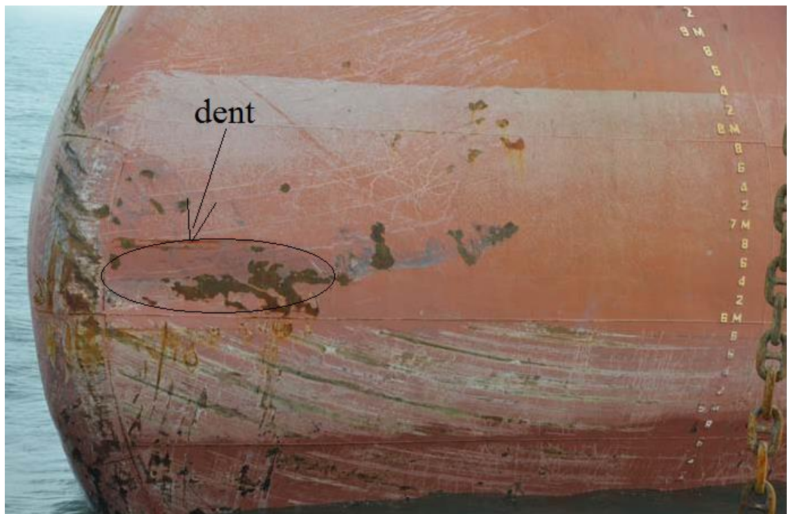
Figure 8- Bulbous bow of Silver Phoenix - a dent length 1500mm, width 500mm and depth 40mm
