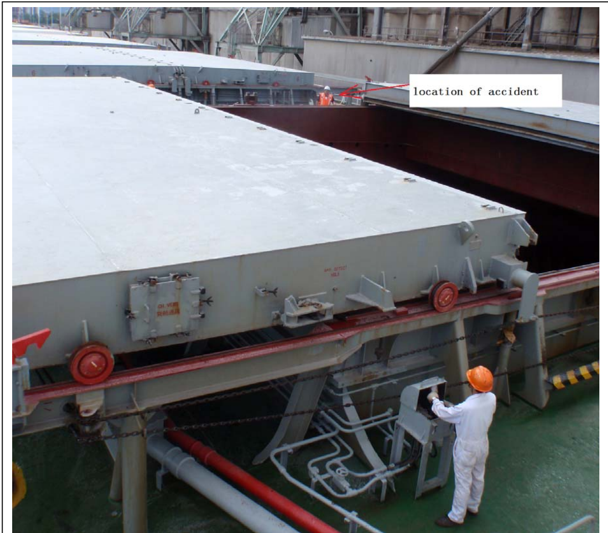
Figure 6- Simulation of the accident: View of operator was obstructed
