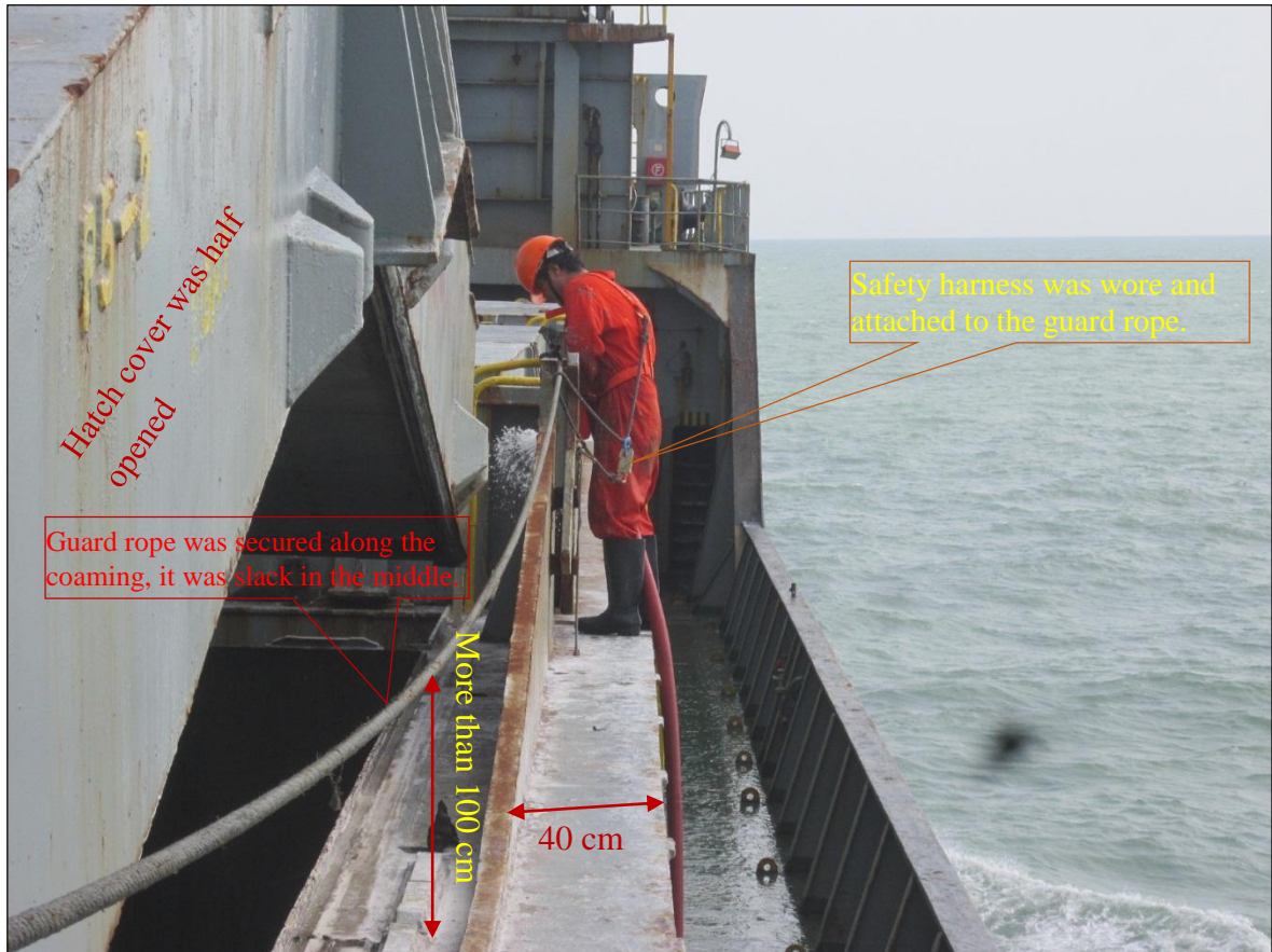
Fig. 4 – One crew was cleansing the hatch coaming on the gutter way.
