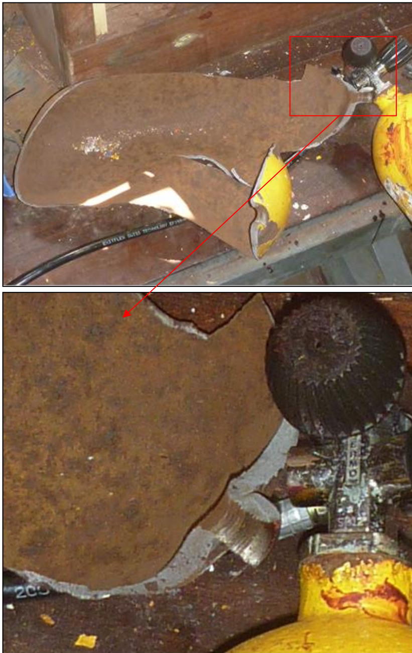
Figure 5: Internal surface of the exploded cylinder was corroded with pitting holes
