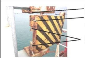
the slot to be plugged in the locking pin to prevent the movement of the platform the handle of the locking pin in lock position
