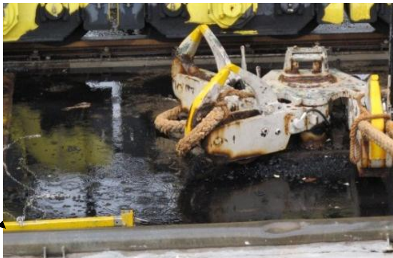
Fig. 6 Rails in ways of the parted rope were knocked out form their anchored positions
