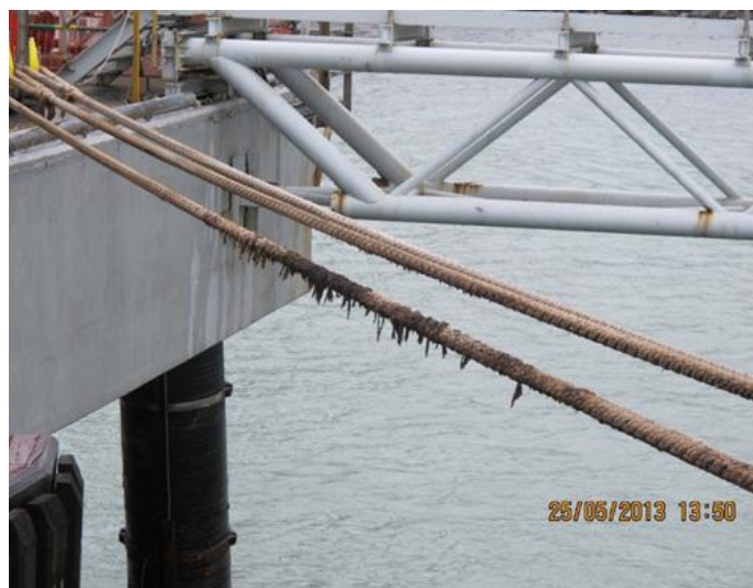
Fig.9 One of the Stern ropes showed sign of chemical damage on the surface
