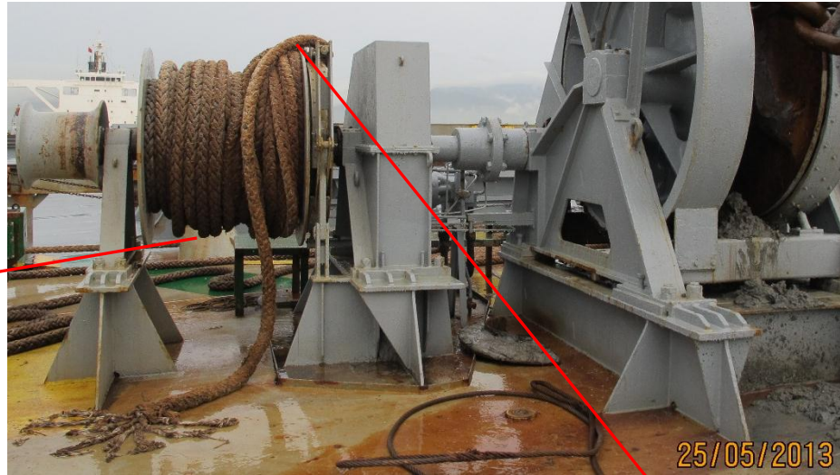
Surface yarns were seriously damaged resulting in a hairy appearance
