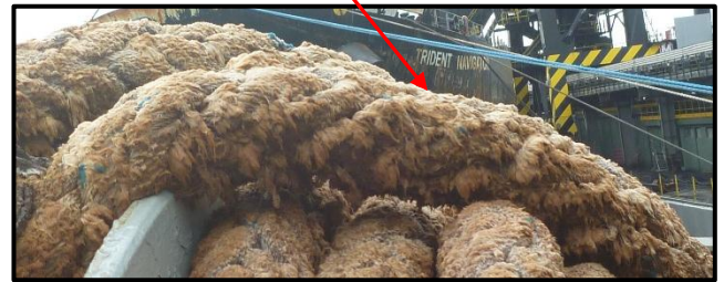
Surface yarns were seriously damaged resulting in a hairy appearance
