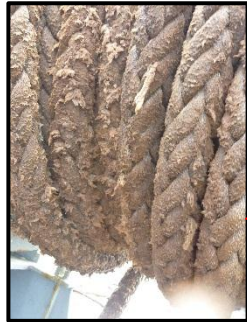
Abrasive wear on the rope
