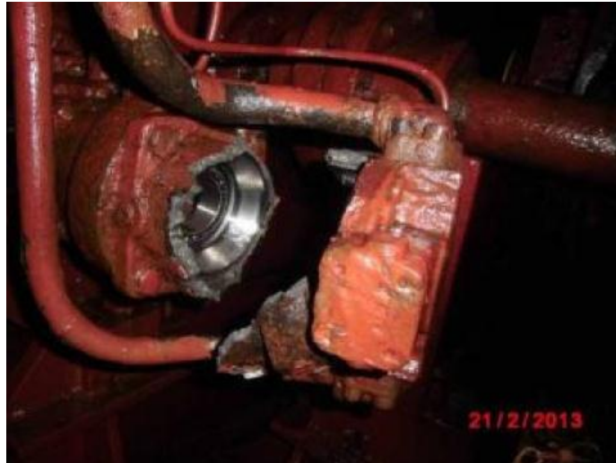
Fig. 5: The damaged port windlass hydraulic motor
