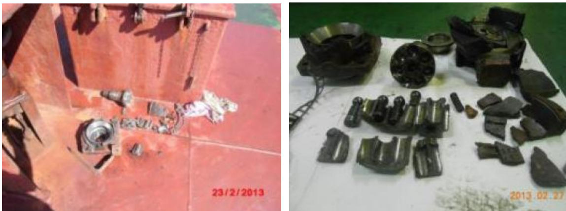
Fig. 6: The broken parts of the port windlass hydraulic motor
