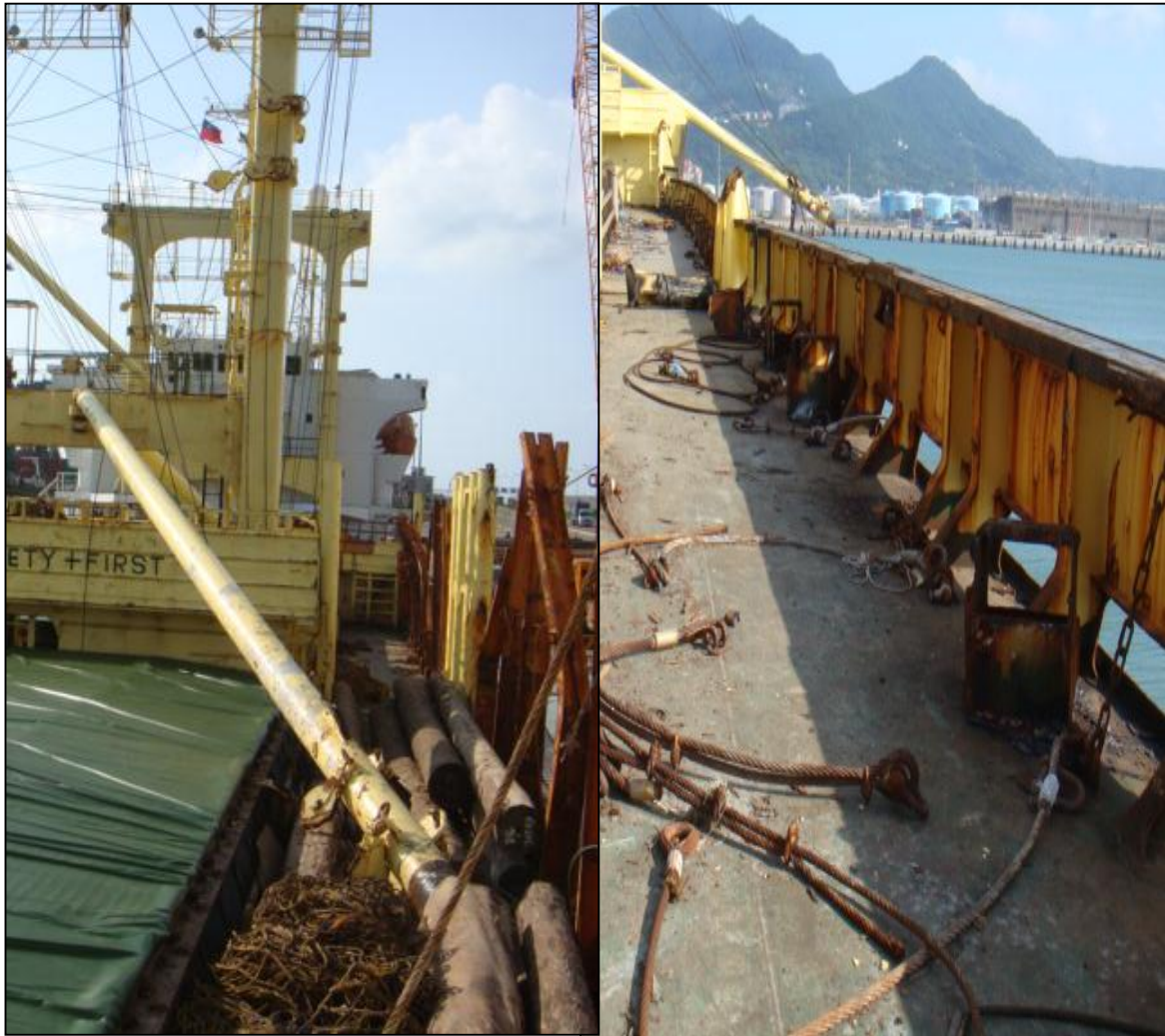
Fig.4 – Bended uprights & collapsed derrick on port side (left), starboard uprights removed (right)
