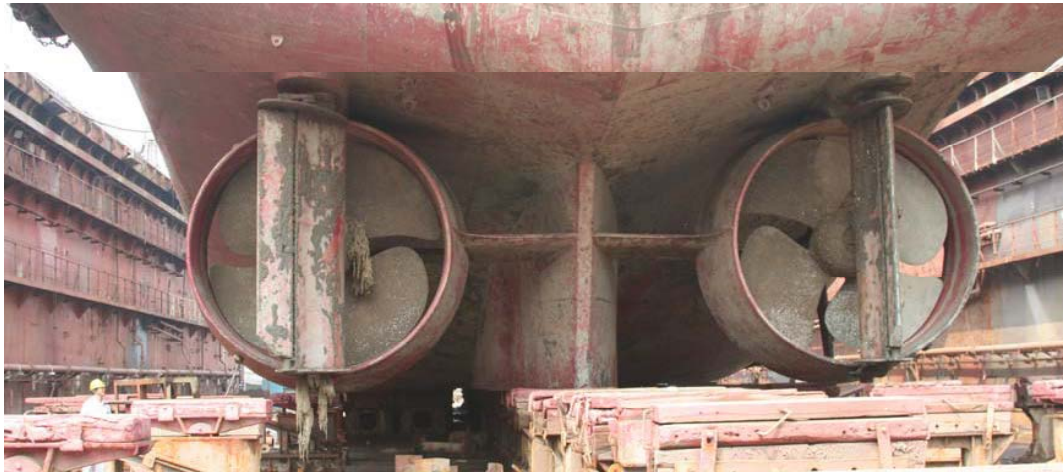
Fig.8 – port propeller was found fouled by a mooring rope.
