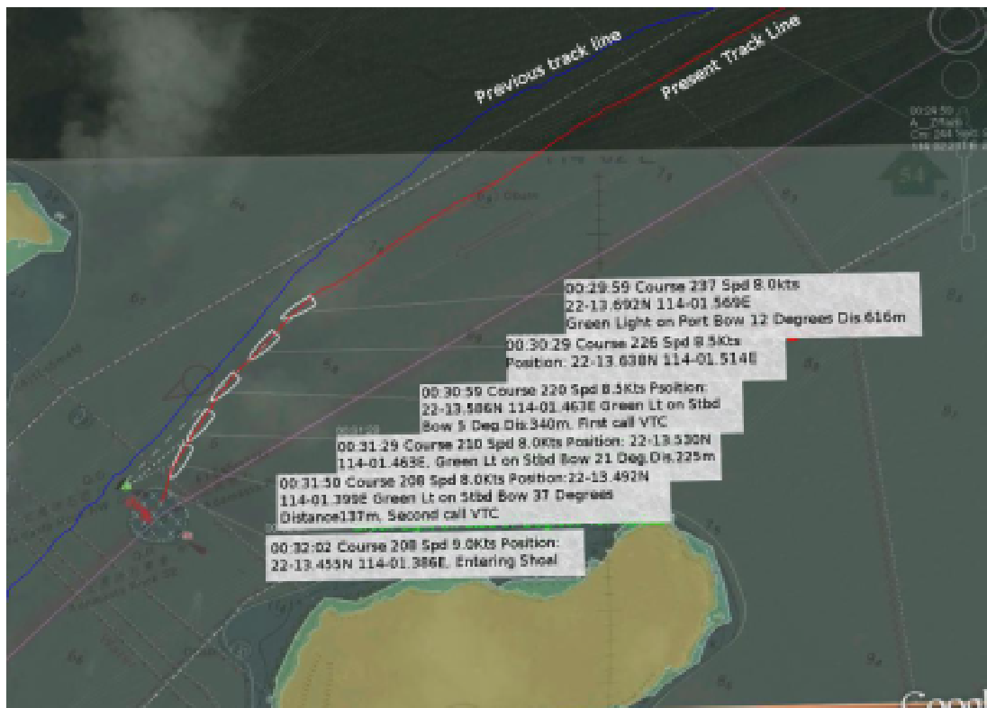
Fig.11 – The movement of ZFFZ running into grounding on the shoal of Adamasta Rock
