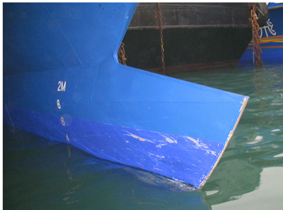
Figure 4 – Scratch marks on the forward port hull of COTAI STRIP COTAIGOLD after collision
