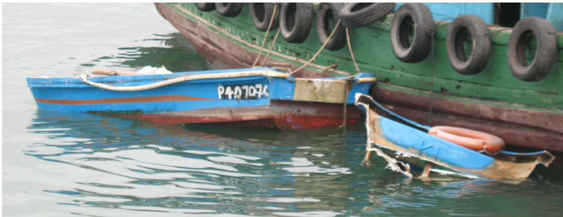
Figure 2- Photograph of P40707C which was broken into 2 pieces
