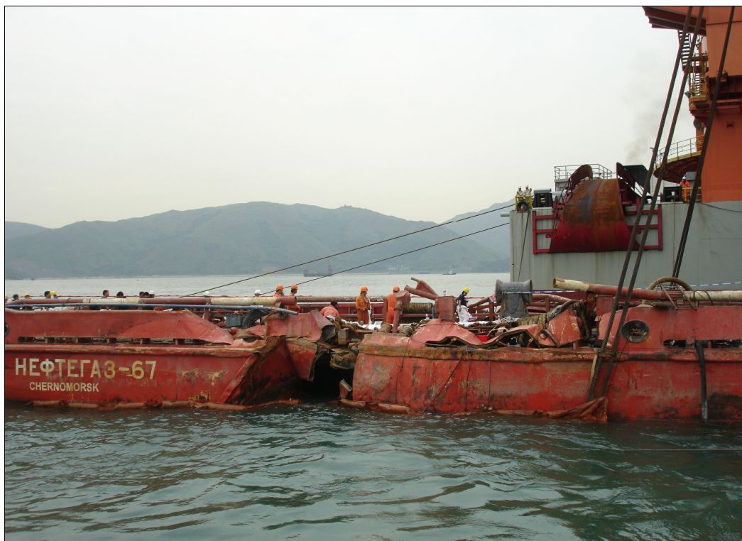
Figure 10-Damage on the starboard side shell of Neftegaz-67
