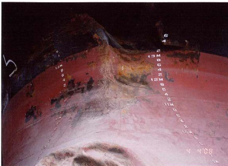
Figure 6B – Damage on stem of Yao Hai
