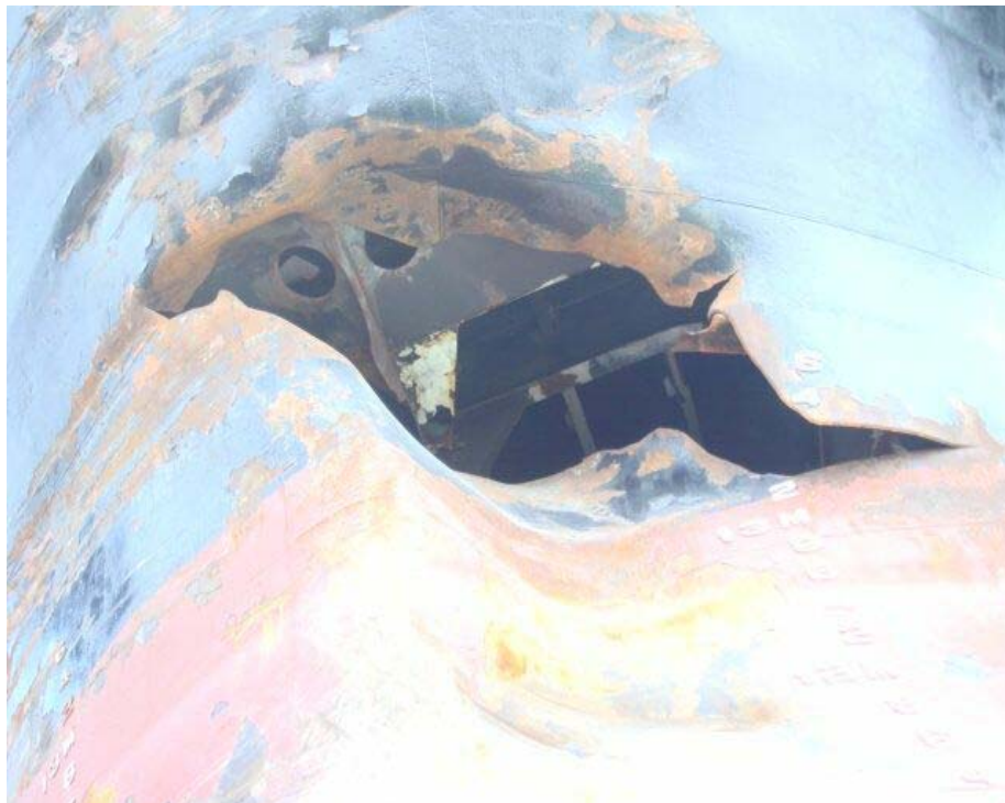
Figure 6A – Damage on stem of Yao Hai
