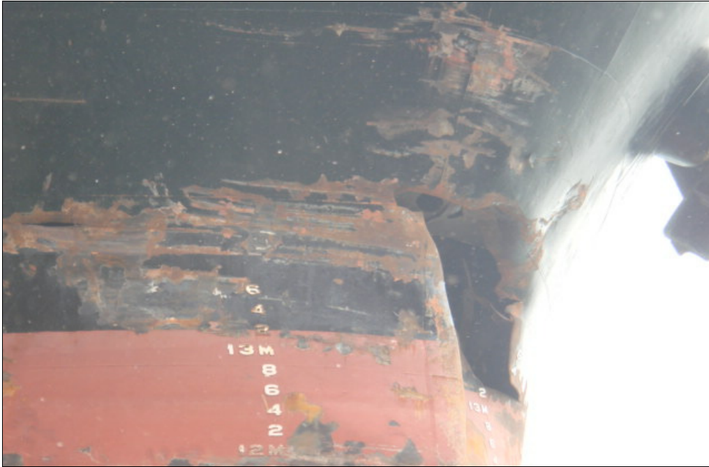
Figure 8- Damage on the stem of Yao Hai
