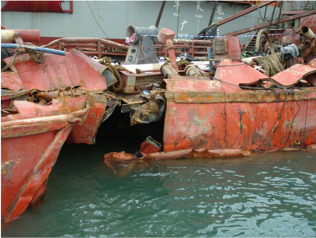
Figure 2B – Damage on starboard side of Neftegaz-67
