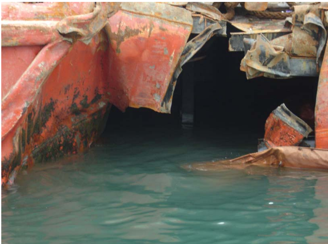
Figure 2C – Damage on starboard side of Neftegaz-67
