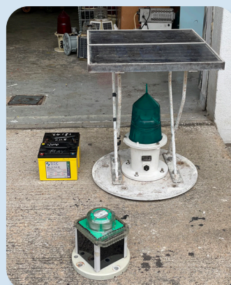
This photo shows a battery (top left), an old version of navigation light equipped with solar panels (top right) and an Integrated Power Supply Lantern (bottom).
