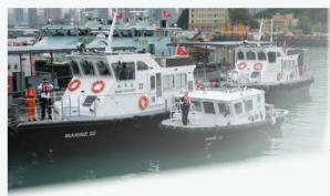
Six new patrol launches have recently joined the Harbour Patrol Section (HPS), including 4 glass reinforced plastic (GRP) launches, namely Marine 18, 20, 21 and 22, with length of approximately 15m, and 2 aluminum alloy catamarans, namely Marine 113 and 115, with length of approximately 10m. They are built in new layouts and equipped with new features to help MD officers enhance marine traffic control.
