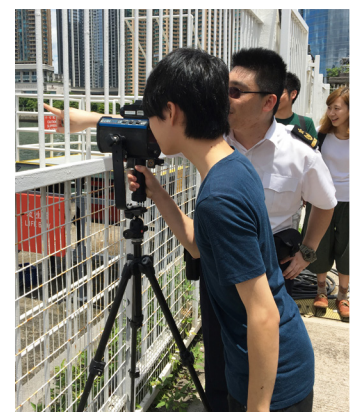
A student is learning to check the speed of vessels with a laser gun.
