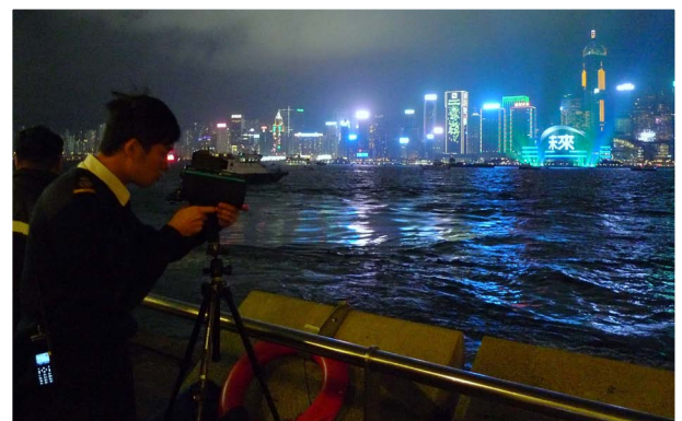
An MD officer checks the speed of vessels with a laser gun to deter speeding.
