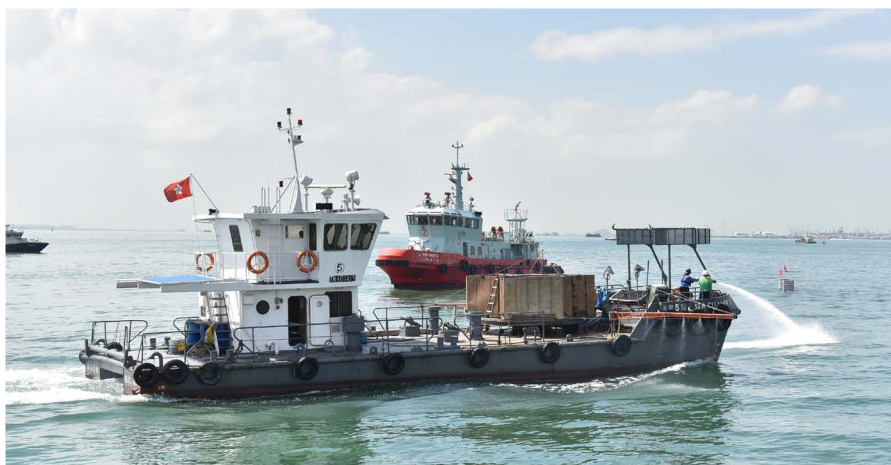
A pollution control vessel sprays sea water onto the sea to simulate the dispersal of an acidic plume and expediting the dilution of phosphoric acid solution.
