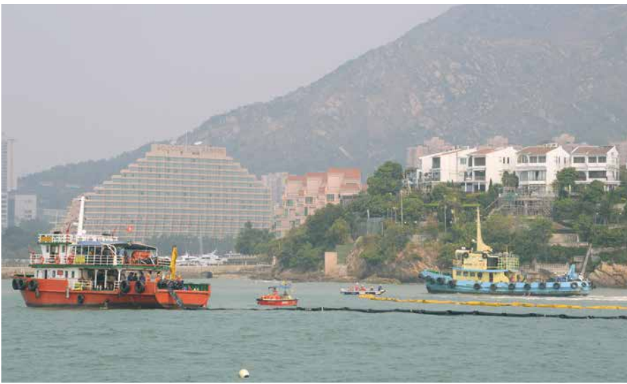
The Marine Department holds two annual marine pollution response joint exercises, code-named Oilex 2014 and Maritime Hazardous and Noxious Substances Exercise 2014, simultaneously off Tuen Mun. Photo shows oil combat teams using floating barrier booms to prevent the simulated spill from drifting.
