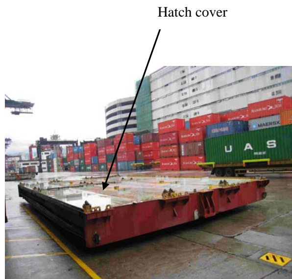
Fig.5: A Hatch Cover Placed at Shore
