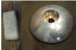
The zinc block is common type of sacrificial anodes
