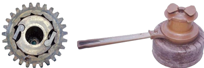
Rope winch — the pawl limits the gear to rotate in single direction only (anti-clockwise)
