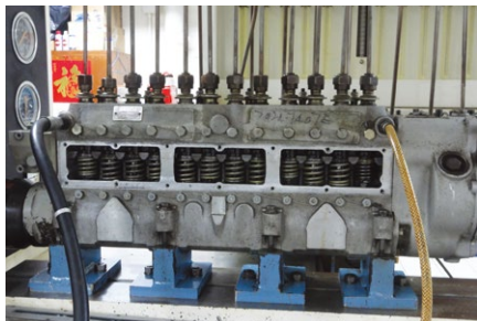
The high pressure fuel pump of diesel engine (for 12 cylinders) is commonly known as flush pump
