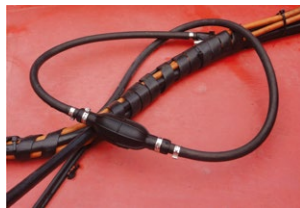
Hand primer bulb in flexible fuel hose
