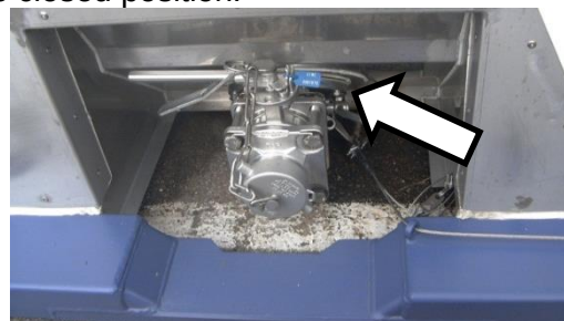
Figure 9.17 Discharge valve seal
