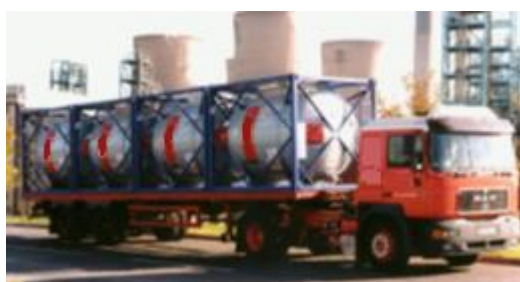
Figure 3.40 – Four 10-foot ISO beam tanks
