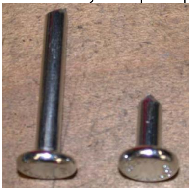
Figure 9.31 Cut bolt seal – stems
