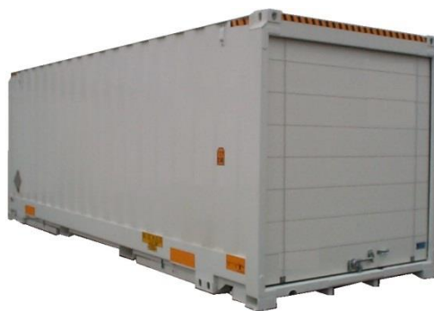
Figure 3.59 – 7.45 Class C stackable swap body with set-back top fittings
