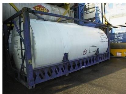
Figure 3.37 – 25,000 l frame tank
