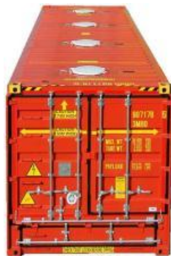
Figure 3.42 30-foot dry bulk box container
