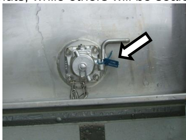
Figure 9.16 Top valve seal
