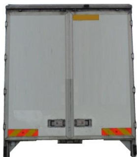
Figure 9.2 Swing door (Road vehicle)
