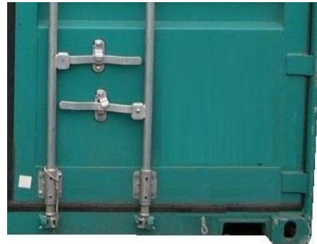
Figure 5.27 Handles between bars
