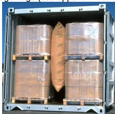
Figure 7.9 Gap filled with a central dunnage bag
