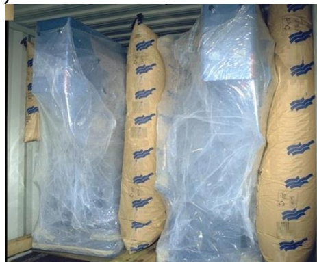
Figure 7.10 Irregular shaped packages blocked with dunnage bags
