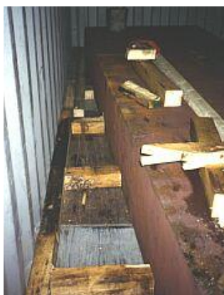
Figure 7.45 Transverse blocking of steel slab
