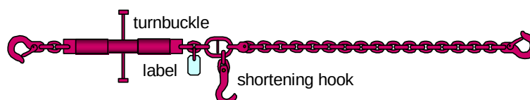
Figure 7.18 Standard chain lashing with shortening hook
