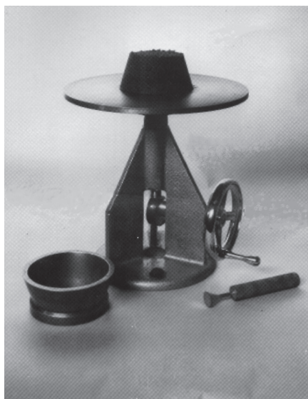
Figure 1.1.2 – Flow table and accessory apparatus
