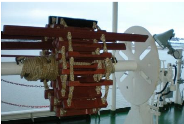
Fig. 3 – Pilot ladder reel
