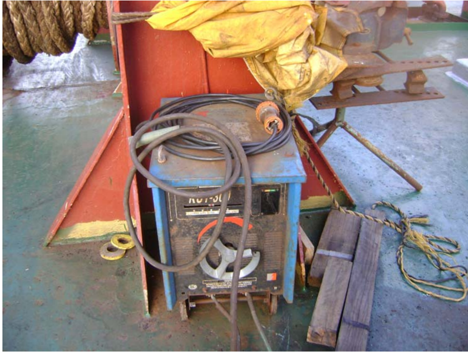
Figure 6 – Portable welding machine used by Fitter A
