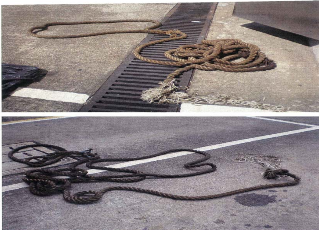
Fig. 2 Parted Stern Mooring Ropes
